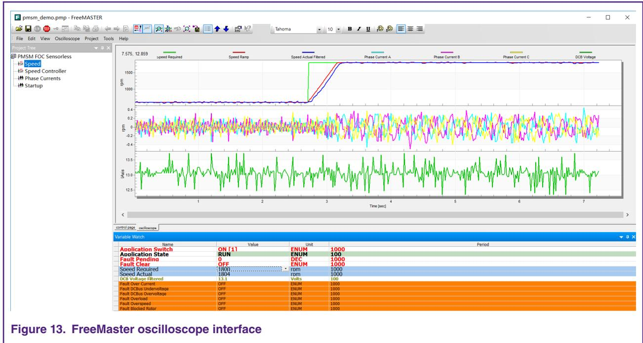
Figure 13. FreeMASTER oscilloscope interface
