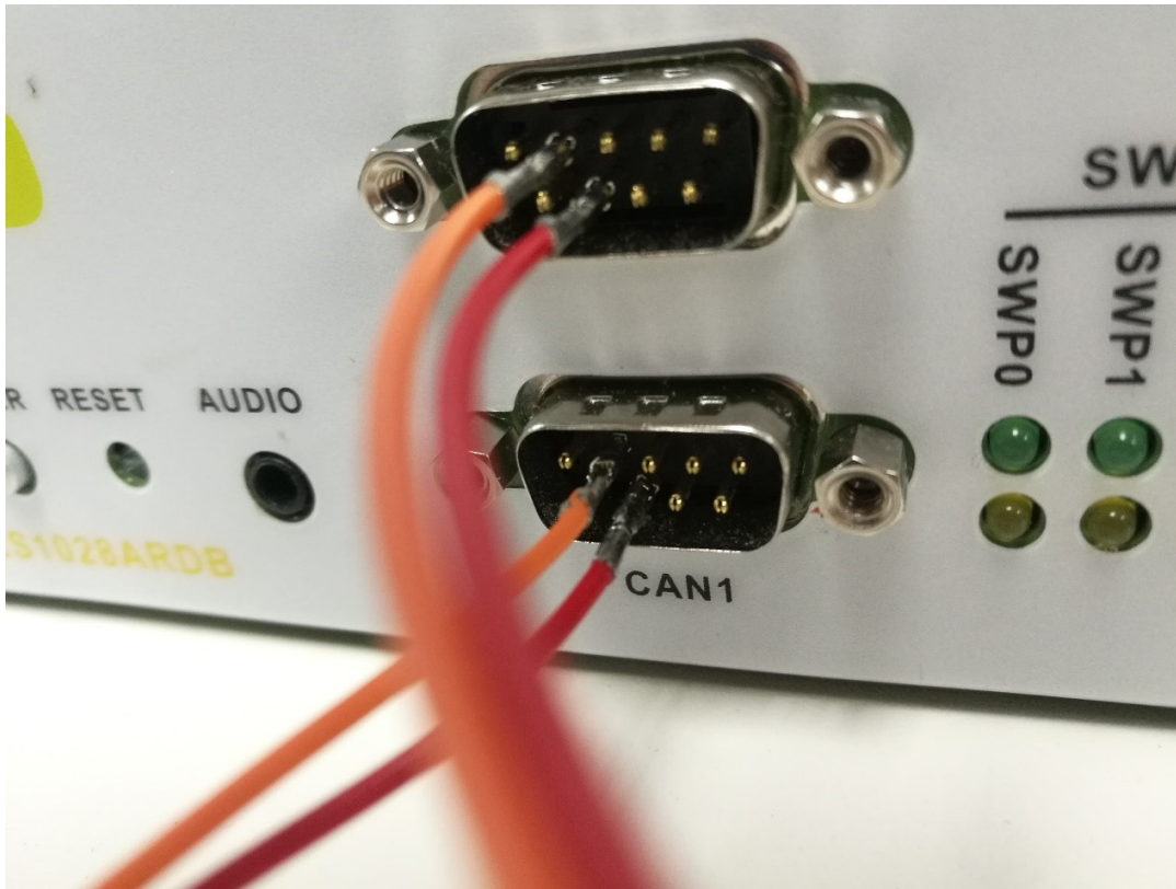
Figure 45. Physical connection for CAN using LS1028ARDB
