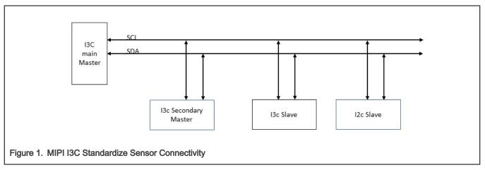
This application note describes how to use the LPC553x/LPC55S3x I3C controller as a master, take full advantage of some key features of the I3C such as DAA and IBI, how to build a sensor network, and communicate with these slave sensors on the network.
